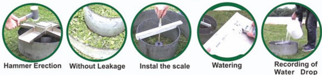
Figure 2: Instalation of double ring infiltrometer.
