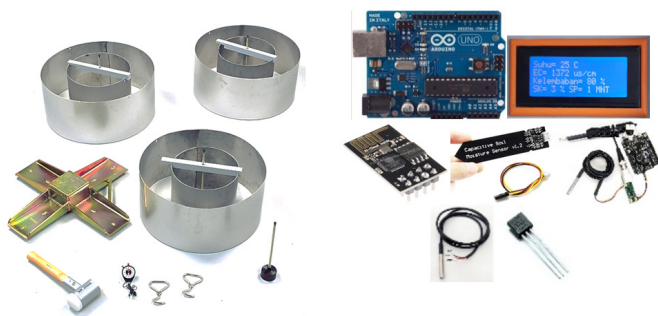
Figure 1 A: Double ring infiltrometer and sensors
