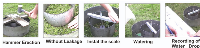
Figure 1 B: Installation of double ring infiltrometer
