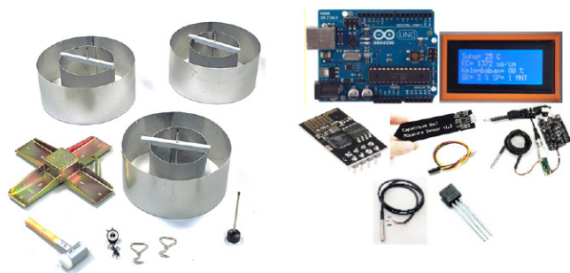
Figure 1A: Double ring infiltrometer and sensors
