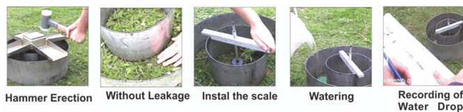
Figure 1B: Installation of double ring infiltrometer
