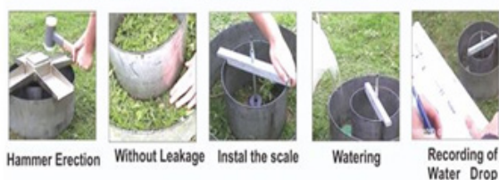
Figure 1B: Instalation of double ring infiltrator
